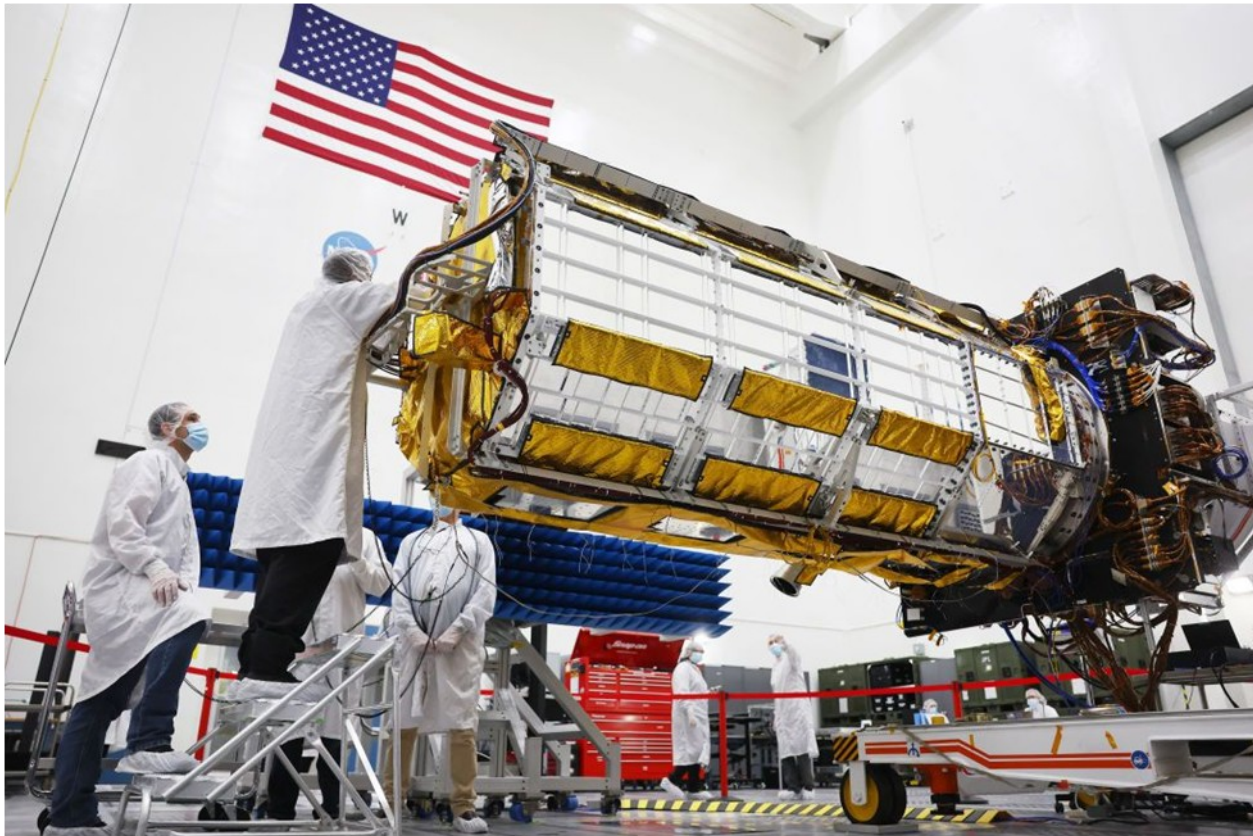
The NASA-ISRO Synthetic Aperture Radar satellite inside a clean room at NASA's Jet Propulsion Laboratory in Pasadena, California. PHOTOGRAPH: MARIO TAMA/GETTY IMAGES
