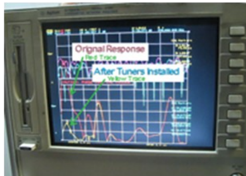
Figure 1. A network analyzer display shows the effects of installing a tuning section of transmission line.
