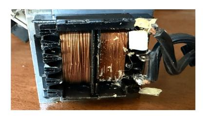
This is one of those "power bricks" that all your gadgets use to plug into a wall socket. The two coils are side by side, and you can see that the one on the right has more "turns" than the one on the left. So, if you have a 120-volt AC input, the output will be lower (in this case it's 12 volts). There's some other stuff in there that takes that lower-voltage AC and turns it into a DC output; that's called a voltage rectifier.
